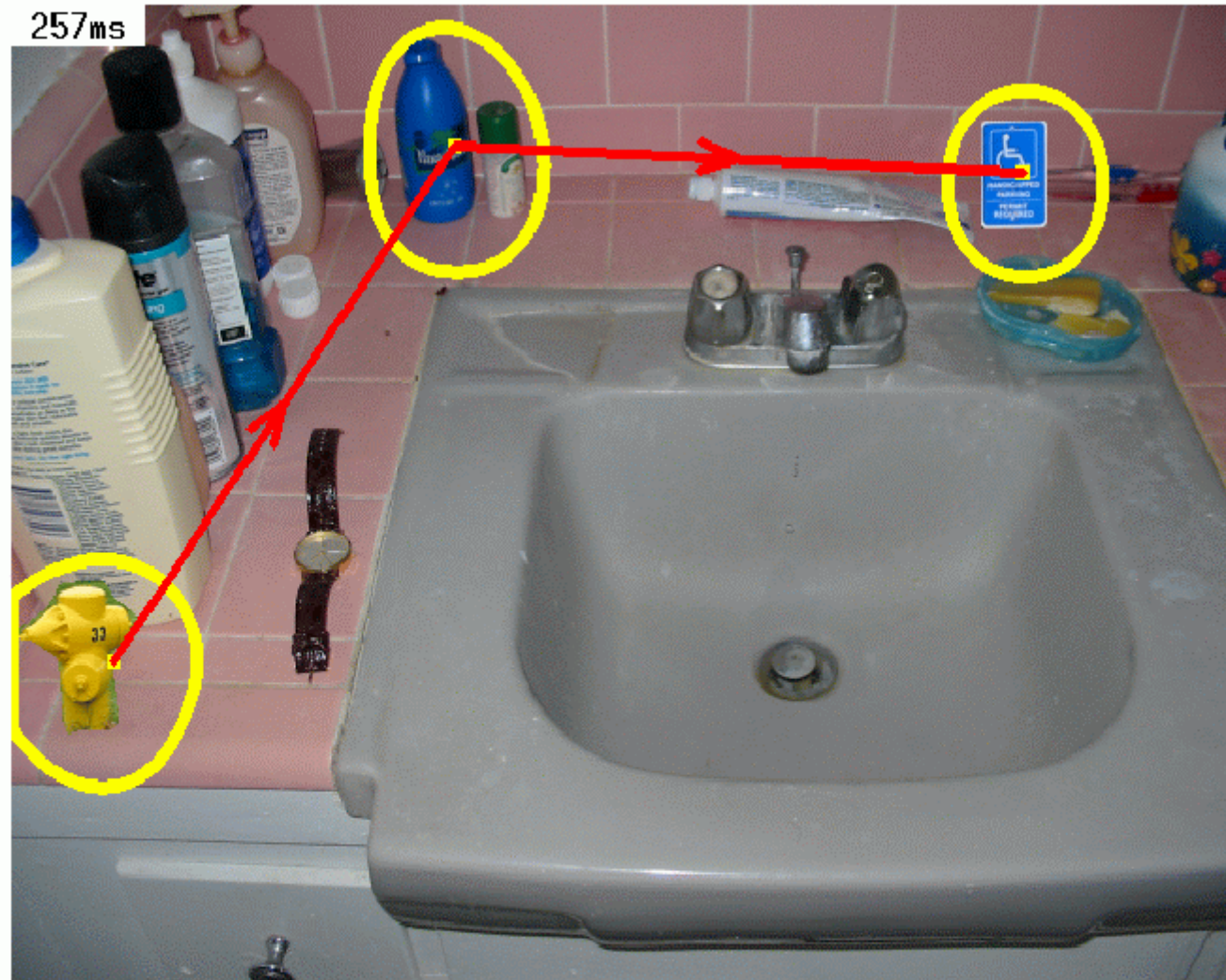
Figure 12: Sequential detection of multiple targets: The model initialized the working memory with the targets to be found and their relevance (handicap sign, relevance = 1; fire hydrant, relevance = 0.5). It biased for the most relevant target (in this case, the handicap sign), made a false detection, recognized the fixation (fire hydrant), updated the state in its working memory (recorded that it found the fire hydrant), and proceeded to detect the remaining target by repeating the above steps.
